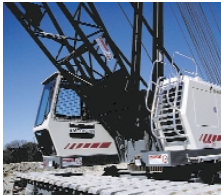
Extra wide cab is set forward of boom foot
